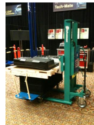
(Stacker removing battery & pallet from Lift Table)
